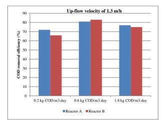
Figure 6: COD removal efficiency of the reactor A (MH A) and reactor B (MHB) at different organic loading rate and the same velocity of 1.3 m/h
