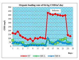
Figure 4: Varying of COD in the influent and effluents from the reactor A (MH A) and reactor B (MH B) at organic loading rate of 0.6 kg COD/m<sup>3</sup>.day
