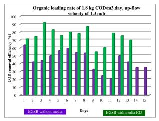
**Figure 7:** COD removal efficiency of the EGSG with and without media F25 at the organic loading rate of 1.8 kg COD/m<sup>3</sup>.day and the up-flow velocity of 1.3 m/h
