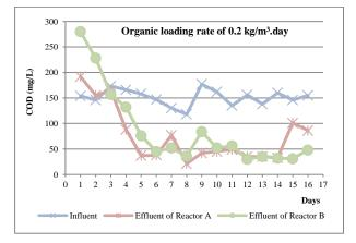
Figure 3: Varying of COD in the influent and effluents from the reactor A and reactor B at organic loading rate of  $0.2 \text{ kg COD/m}^3.day$
