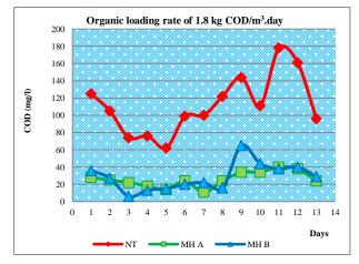
Figure 5: Varying of COD in the influent and effluents from the reactor A (MH A) and reactor B (MHB) at organic loading rate of 1.8 kg COD/m<sup>3</sup>.day
