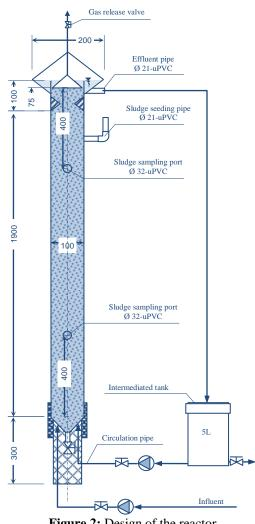
Figure 2: Design of the reactor
